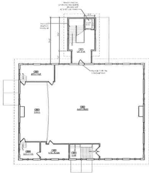
EXISTING ASSEMBLY USE COULD STAY ON 3RD FLOOR LEVEL NOTE: STATE MAY REQUIRE THAT A SPRINKLER SYSTEM BE INSTALLED AND/OR OCCUPANCY ON 3RD FLOOR LIMITED TO LESS THAN 300
