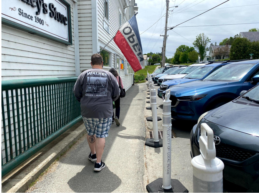
Above: Bollards were placed along the sidewalk in front of Wiley's to simulate wheelstops and keep drivers from blocking the sidewalk.
