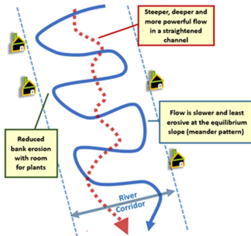
Figure 1 River Corridor Diagram showing room for river channel adjustments to minimize slope and erosive power.
